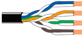
Figure 9 Typical twisted pair cable
